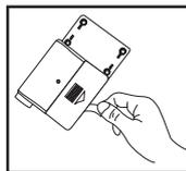
Remove the battery isolator
